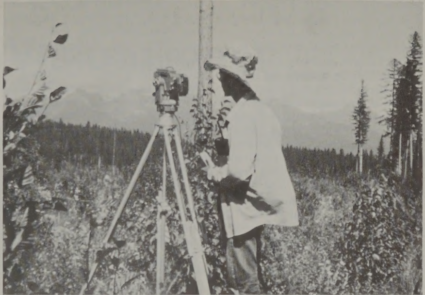
Theodolites and laser range poles add to the capabilities of magnetic and solar compasses.
